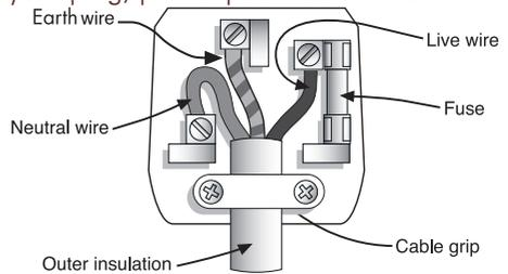
The wire coloured BLUE is the NEUTRAL and must be connected to the terminal marked N or coloured BLACK.
